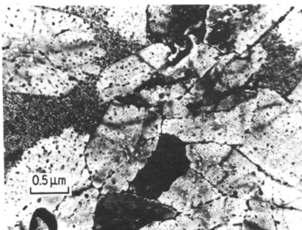
Figure 12 Electron micrograph of the \alpha - \text{Al}_2\text{O}_3 film obtained by annealing at 1520 K for 5 h. In the picture areas of fine crystalline \delta - \text{Al}_2\text{O}_3 can be seen.
